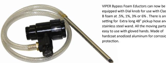
equipped with Dial knob for use with Class A or B foam at .5%, 1%, 3% or 6%. There is an off setting for Extra long 48" pickup hose and stainless steel wand. All the moving parts are easy to use with gloved hands. Made of hardcoat anodized aluminum for corrosion
