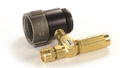
Designed to protect hose lays from pressures beyond requirements. This valve is installed at any point in a 1 ½"/38mm discharge hose lay and will automatically reduce excess pressures via an adjustable, automatic pressure bleed off 3/4"/19mm Male GHT outlet. This is designed to allow the attachment of a 3/4"/19mm Myti-Flo® hose to keep the area dry. Aluminum, brass and stainless steel construction. Connections are available in NPSH, NH and QC. Other options are also possible.
