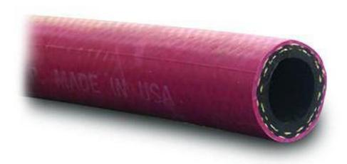
Multipurpose is an EPDM hose designed for continuous flow hose reels. It's our toughest and most durable non-collapsible hose. The EPDM tube and cover, reinforced with polyester yarn allows Multipurpose to be used in a variety of environments as well as remain fully functional in cold temperatures. Suitable for fire protection or industrial applications. Available in a variety of lengths and sizes (see below).
