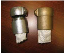
Photo of defective hose coupling. Female Swivels separates under low pressure or fail to rotate as designed.
