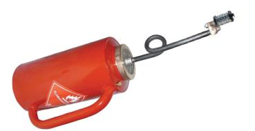
Constructed from light weight and long lasting aluminum with safety features such as a check valve, fuel trap, and a selfextinguishing igniter when the unit is in an upright position. The wand reverses for convenient and leak proof storage within the reservoir. Tank capacity 1 Imp. gal. / 1.2 US gal. / 4.5 L.
