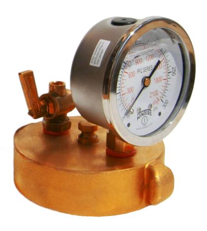
2.5" Brass cap complete with Winters liquid filled gauge, 0-300 Psi. Comes with petcock valve for manual relief of pressure. Available in a variety of hose threads. May be placed directly onto a hydrant to determine static pressure. Please contact your local branch for availability.
