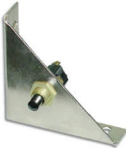
**CMS-01:** Monitor switch with mounting bracket. Designed to sound an alarm or signal a panel in the event the cabinet door is opened. Constructed of 18 gauge metal with a Nickel Chrome plating for added corrosion resistance. Electrical monitor switches can be installed on all National Fire Equipment's Cabinets. (Alarm, Alarm Panel and Electrical Wiring Not Included)
