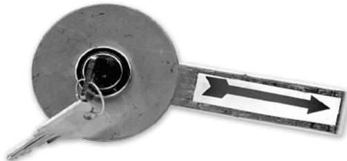
**BGL-87127:** Break Glass Lock Assembly can be provided on all NFE's fire protection cabinets. Provided with 2mm break glass on full metal doors or with 3/16" (5mm) scored glass on full glass fronts. Emergency access is gained by shattering the glass and pulling the inside lever. Recommended for installation at the factory but is also available for site installation. Comes complete with instruction decals.
