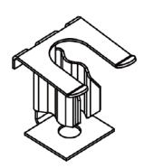
Function: Designed to restrict the upward movement of activated fire sprinkler
