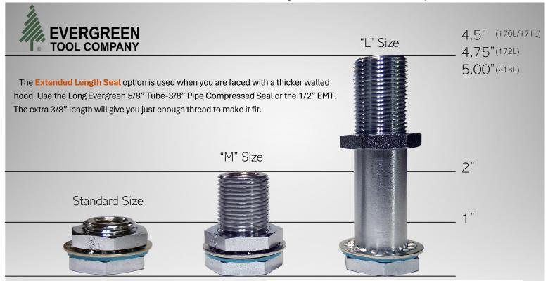
We offer a full line-up of 3/8" through 1" Extended Length Quik-Seals. The "M" size is made for hoods that need just a few more threads. The "L" length Seal has even more threads and designed for dry chemical systems like paint spray booths.
