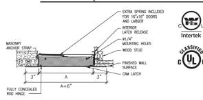
Warnock Hersey International, Pittsburgh, CA 3 Hour. rating for noncombustible floor/ceiling assembly, Report# WHI-495-PSH-0192. These doors may be used in a 2-hour fire rated wall assembly. For fire rated ceilings, this door has been approved by Warnock Hersey International for 3 hours (\*max. size to 24" x 36").
