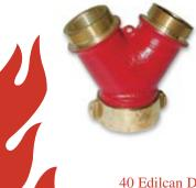
Application: For dividing one supply line into two separate lines.Construction: Available in cast brass or lightweight cast aluminium. Female Hose Thread Inlet x (2) male hose thread outlets
