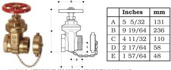
WARNING: NOT DESIGNED FOR FIRE DEPARTMENT STANDPIPE VALVE Use Model A86 soft seated valves only for FDC Connections fire hose cabinets & standpipe risers. Application:Used for standpipes, fire pumps and<br/>hydrants as a control shut off valve.Construction:Forged brass body with red hand wheel,<br/>solid brass wedge disc with tapered seats.Rated Pressure:300 psi / 2069 kpaApprovals:UL & FMOptional Finishes:A53B – Rough BrassA53B – Polished BrassA53PC – Polished Chrome
