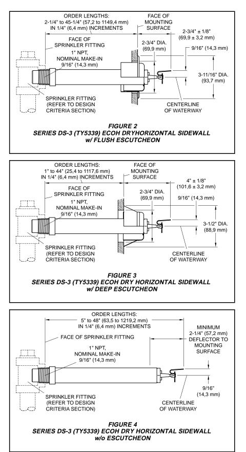
the appropriate length of the sprinkler that will prevent freezing of the water in the connecting pipes due to conduction. When the temperature surrounding the wet pipe sprinkler system is maintained at a minimum temperature of  $40^{\circ}$ F/4°C, the following are the minimum recommended lengths between the face of the sprinkler fitting and the outside surface of the protected area (i.e., length exposed to minimum ambient of  $40^{\circ}$ F/4°C):
