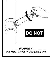
valve must be closed and the system drained before removing the sprinkler.
