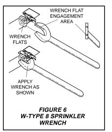
the sprinkler into the sprinkler fitting.
