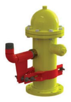
Hydrant Mount 2-1/2" (64mm) or 3" (76mm) NPT male discharge thread with 2-1/2" (64mm) NH female swivel inlet. "C" clamp hydrant bracket support arms are designed to fit on virtually any hydrant style. Red epoxy finish.
