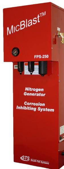
The MicBlast™ is designed to supply low pressure, supervisory Nitrogen, a clean, dry, non-flammable, inert gas to pre-action and dry sprinkler systems. Traditionally compressed air is used as a supervisory gas for such systems. However, the constant availability of oxygen in the compressed air supports corrosion of the steel and galvanized piping. Microbiologically influenced corrosion (MIC) has also been identified as a real threat for the integrity of these types of fire protection systems.
