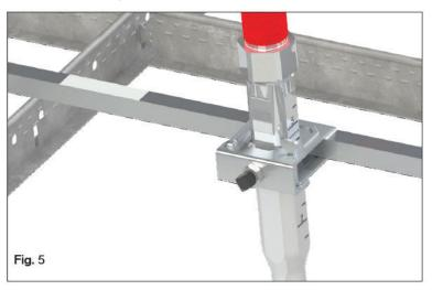
7. Ceiling tile Installation- The flexible sprinkler drop system with IPT bracket is able to be installed prior to the ceiling tile installation, preventing the need for sprinkler contractor tile adjustment. For ease of tile installation, cut the largest sprinkler hole recommended by sprinkler head manufacturer. The largest hole that is still covered by the sprinkler escutcheon allows for
