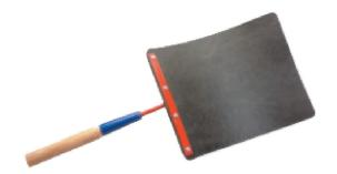
Used mainly for smothering and extinguishing grass fires, Fire Swatters are also used for "mopping up" after brush fires. Field tested and proven over many years. The 12" W x 15" L rubber flap is first attached to a steel frame, then secured to a 60" ash handle with ferrule.
