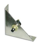
CMS-O1: Monitor switch with mounting bracket. Designed to sound an alarm or signal a panel in the event the cabinet door is opened. Constructed of 18 gauge metal with a Nickel Chrome plating for added corrosion resistance. Electrical monitor switches can be installed on all National Fire Equipment's Cabinets. (Alarm, Alarm Panel and Electrical Wiring Not Included)
