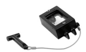
CCC-001: Similar to the Peak Unit, the CCC-001 fits over a standard cabinet latch. Breaking the special break glass with the provided hammer, exposes the cabinet door latch. Constructed of cast aluminum with a red enamel finish.
